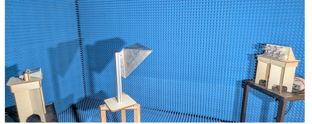
Fig. 2: Software defined radio measurement setup
